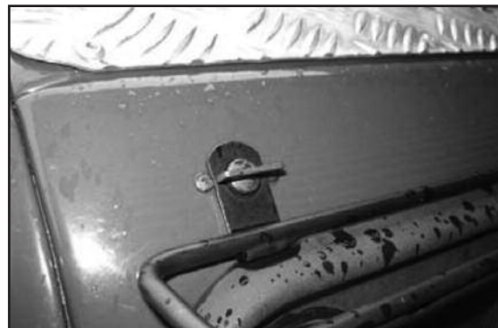
For the 2 larger rectangular light guards use 2 of fixing B as shown in Pic 3 and 2 of fixing A as shown in Pic 4.
