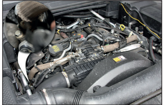
View of engine with top cover removed – right hand EGR valve shown in inset
