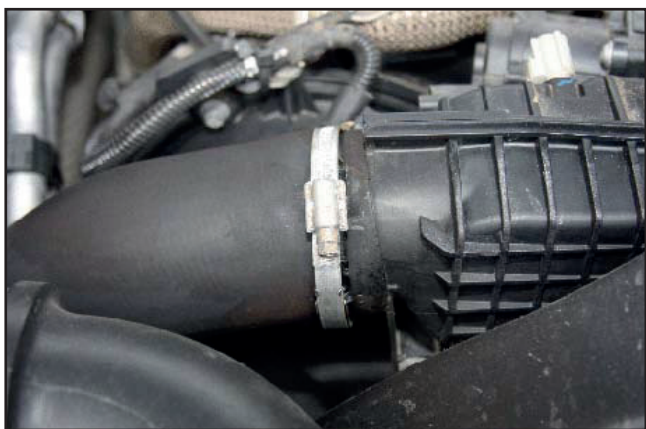
Air inlet pipe to air box jubilee clip
